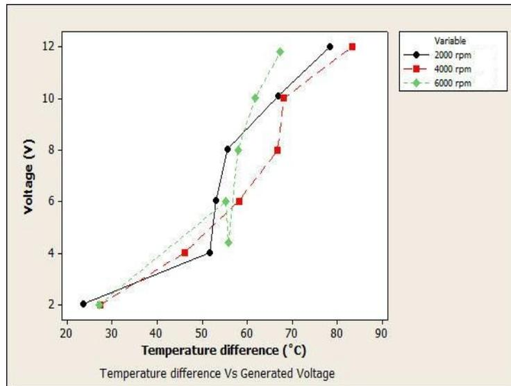
**Figure 12:** Shows that temperature difference is directly proportional to voltage
