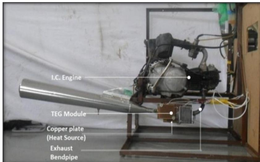
**Figure 10:** Experimental setup of present study
