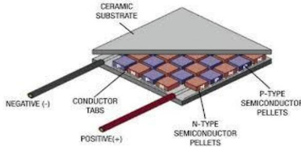
**Figure 2:** Thermoelectric generator [4]
