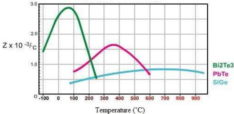
**Figure 3:** Performance of Thermoelectric Materials at various temperatures [4]
