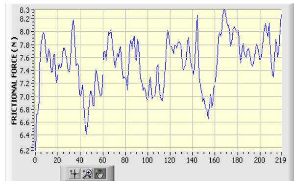
**Fig1.5** Friction vs Distance for 20N load
