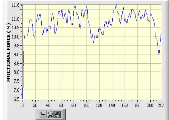
**Fig 1.6** Wear vs Distance for 30N load    **Fig 1.7** Friction vs Distance for 30Nload
