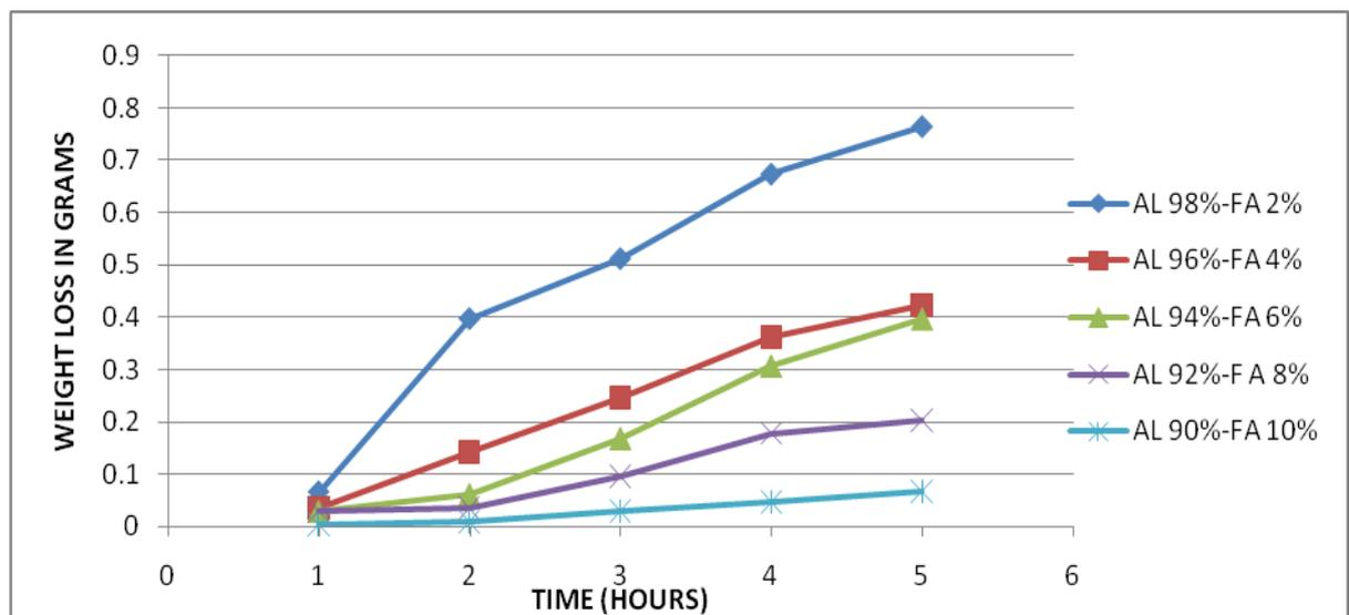
**Fig 1.8** Graphical representation of corrosion rate values
