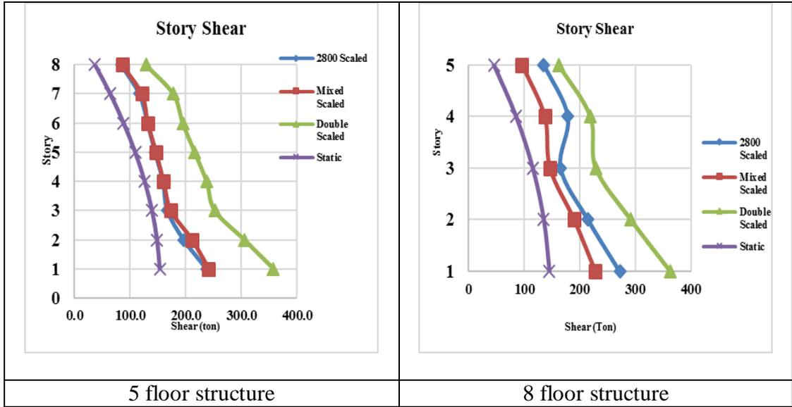
Figure 7: comparison of floor cutting in structures with different methods
