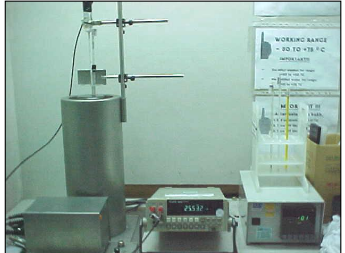
Fig. 2. Set-up for calibration of thermometers by comparison method using a calibration bath.
