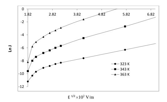
Variation of LnJ versus E  $^{1/2}\times10^2$  V/m for the sample of thickness 1.5  $\times10^{-3}$  m
