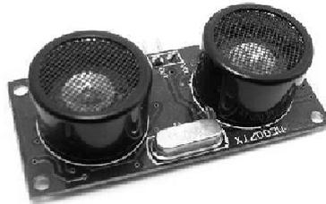
**Fig. 3:** Ultrasonic Transducer Module.
