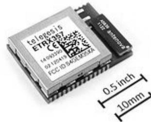
**Fig. 5:** Zigbee hardware module.
