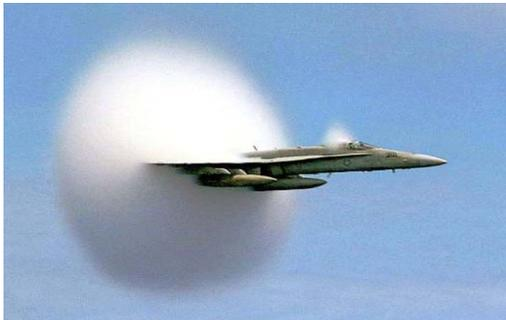
Fig. 1: Shock wave on aircraft [5]
