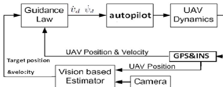
System architecture for visionbased tracking of moving target by an unmanned aerial vehicle
