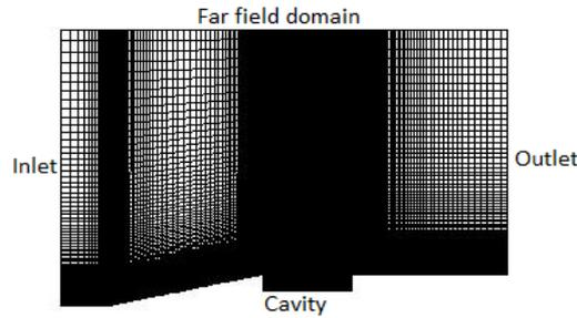
**Figure 2:** Axisymmetric grid for  $L/D=5$
