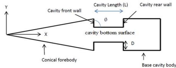
**Figure 1:** Cavity geometry and nomenclature (Sinha et al. 2013).
