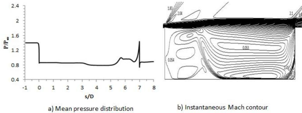
Figure 3: Mean pressure and instantaneous mach contour for  $L/D=5$ .
