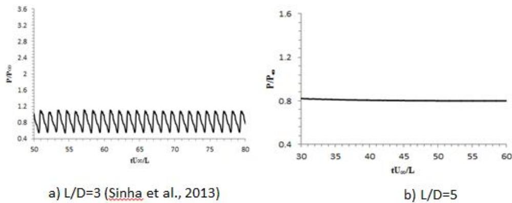
Figure 4: Comparison of pressure oscillation on mid cavity base.
