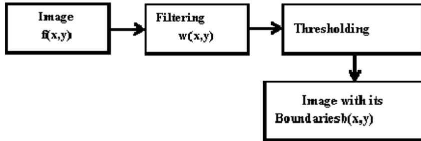
Figure 1: Process flow
