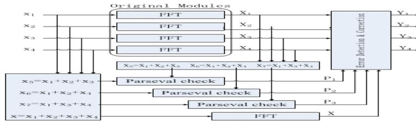
Figure. 3: Parity-SOS-ECC (second technique) fault-tolerant parallel FFTs.
