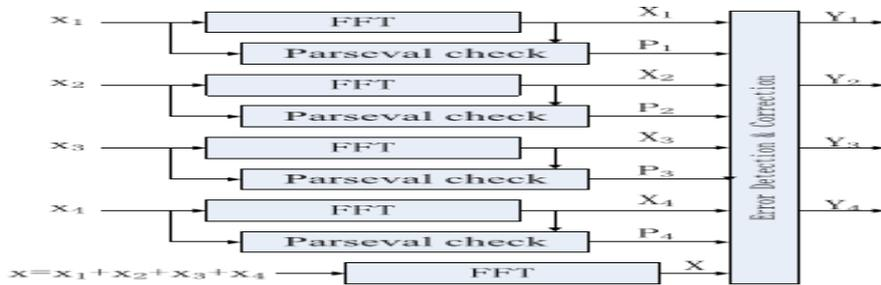
**Figure. 2:** Parity-SOS (first technique) fault-tolerant parallel FFTs.
