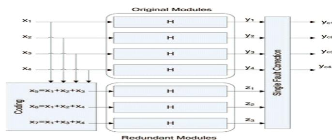
**Figure. 1:** ECC-based scheme for four filters and a Hamming code.
