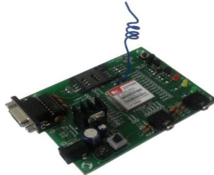
SIM900 GSM module which is extremely popular is used in this project.
