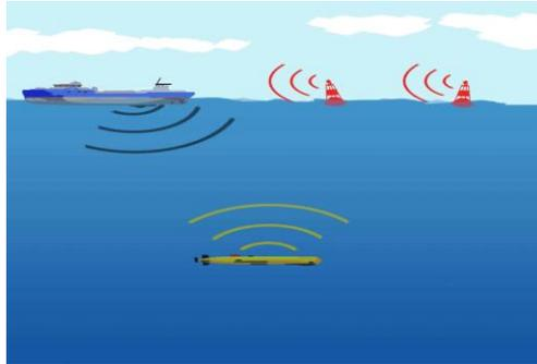
**Fig 1:** Positioning system based on GPS and acoustic signals.
