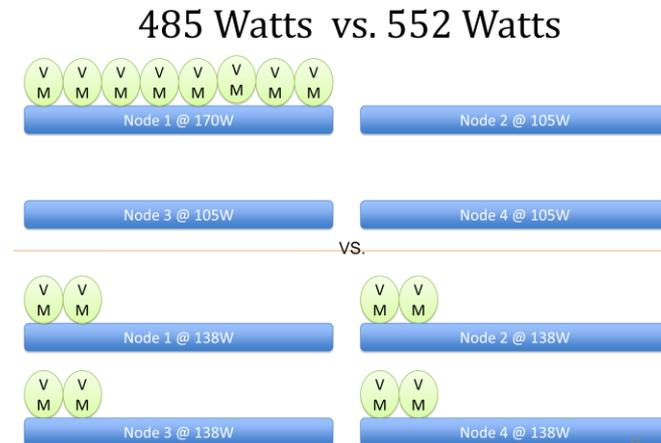
**Fig 2.3** Energy saving through virtualization
