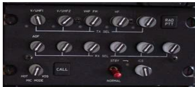
Fig.1.3: Station box in ALH
