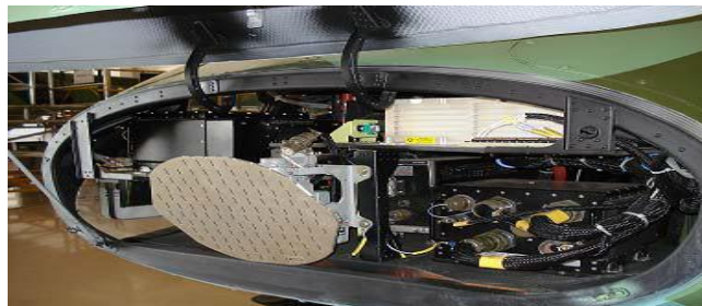
Fig.1.2: Junction box in ALH
