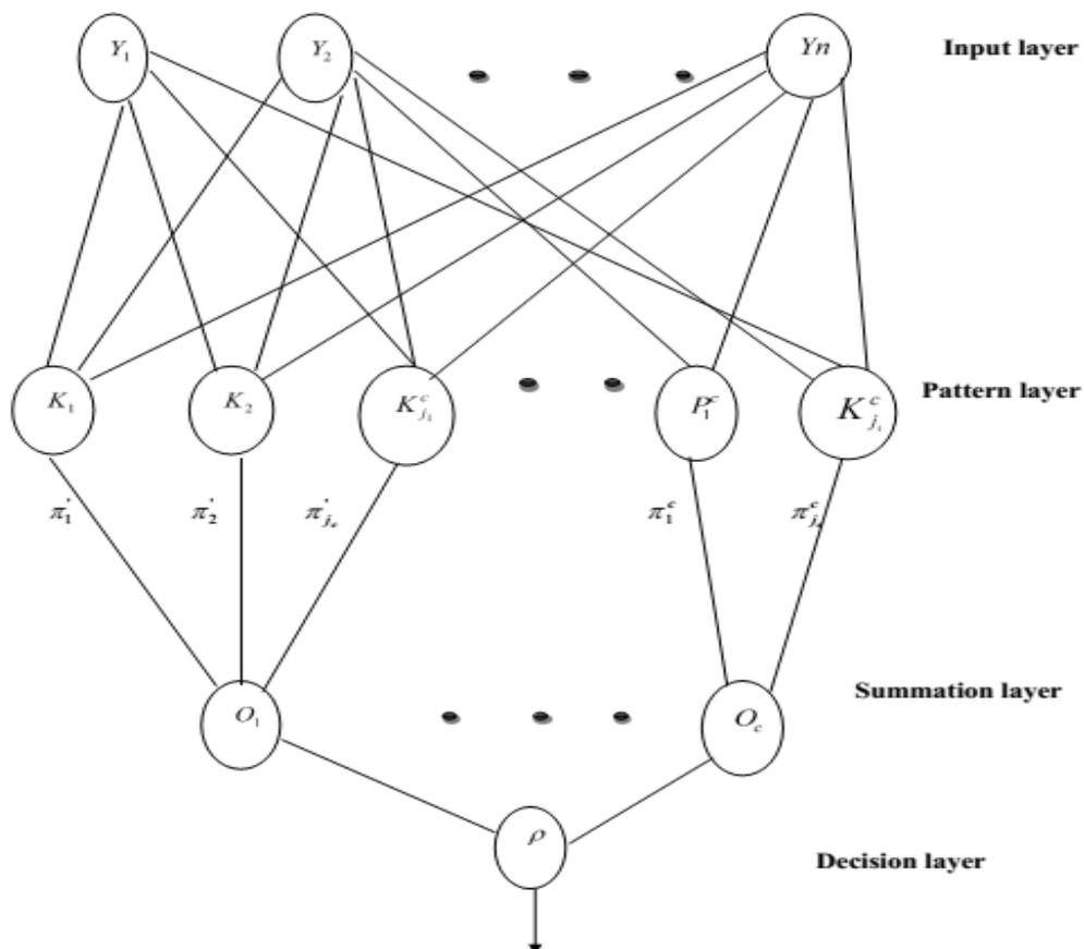
**Fig 3:** Probabilistic Neural Network classifier
