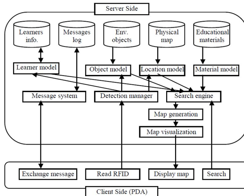
**Fig 5: PERKAM System Architecture**
