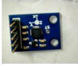
**Fig (d):** Accelerometer sensor view
