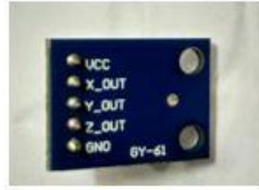
**Fig (e):** Accelerometer connections view
