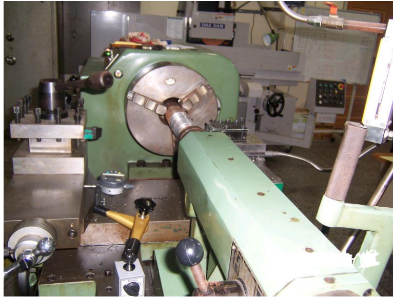
Fig.3 Experimental set-up for finding feed effect on stability
