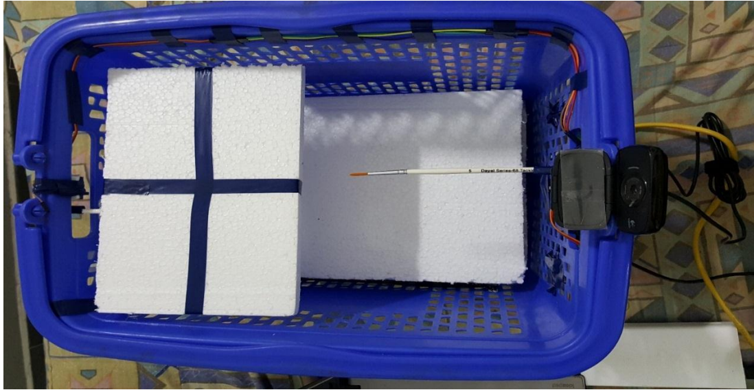
SNAPSHOT 9 - Top view Of The Smart Kart Displaying Servo Motor, Web Camera And The Slab
