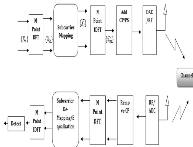
**Figure 1:** Transmitter and receiver structure of SC-FDMA [12]
