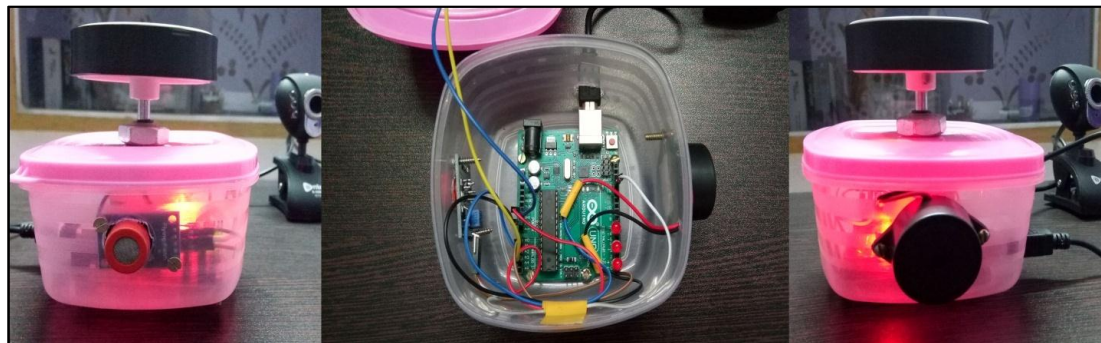
Figure 9 Actuator prototype with alarming system
