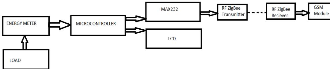
**Fig (a):** Block diagram of the proposed system
