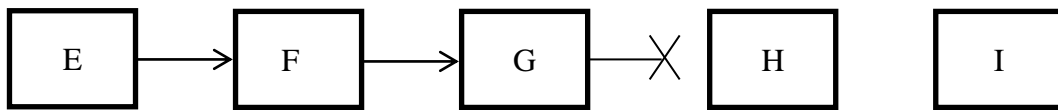
Figure 3: Route maintenance example: In which node G is unable to forward a packet from E to I over its link to another hop H.
