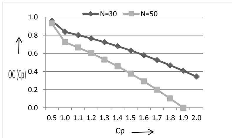
**Figure 3.1:** OC curve for sampling plan that rejects process capability if  $C_p < c$  where  $c=1.33$
