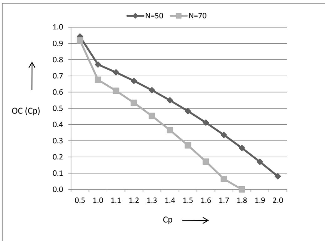
**Figure 3.2:** OC curve for sampling plan that rejects process capability if  $C_p < c$  where  $c=1.46$
