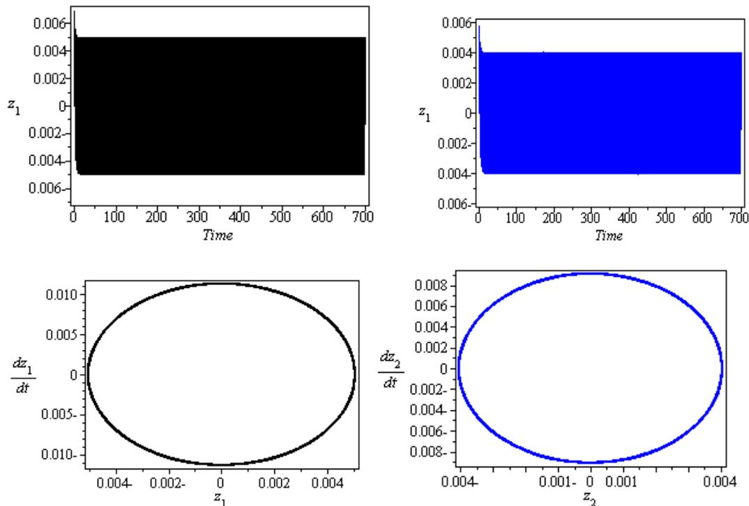
**Fig. 2.** The response amplitude of the vertical shaking conveyor system after control at the case ( $\Omega \cong \omega_n$  and  $\Omega_1 \cong 2\omega_n$ ,  $n = (1, 2)$ ).
