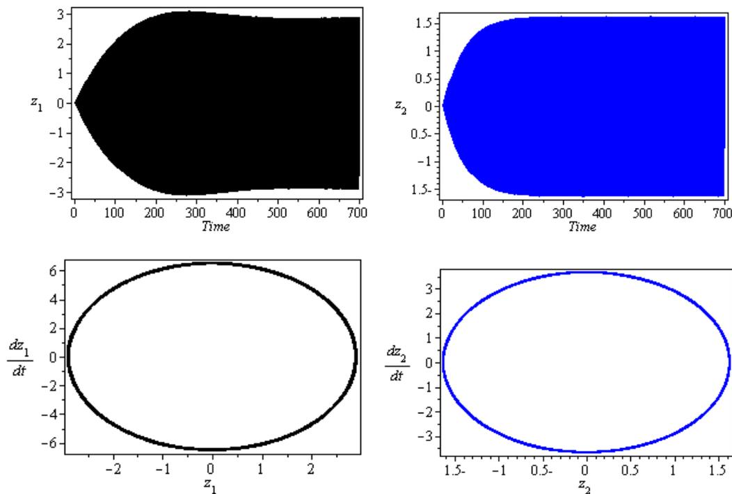
**Fig. 1.** The response amplitude of the vertical shaking conveyor system before control at the case ( $\Omega \cong \omega_n$  and  $\Omega_1 \cong 2\omega_n$ ,  $n= (1, 2)$ ).
