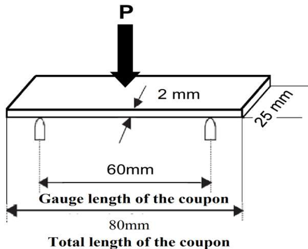
**Figure 7:** The configuration of the flexural test setup with the coupon
