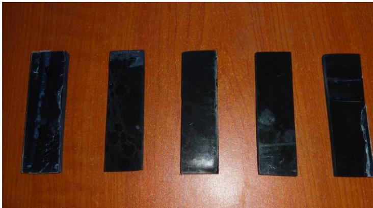
**Figure S.1:** Digital image of flexural coupons (dM-CP) obtained from direct-mixed CNF/ER composites
