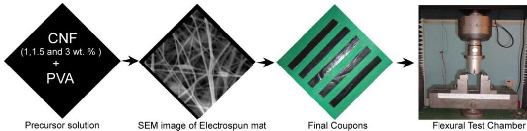
**Figure 5:** Schematic illustration describing the steps involved in fabricating flexural coupons and their mechanical testing
