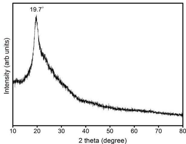
**Figure 9:** XRD pattern shows semi crystalline nature of the CNF/PVA nanofiber mats
