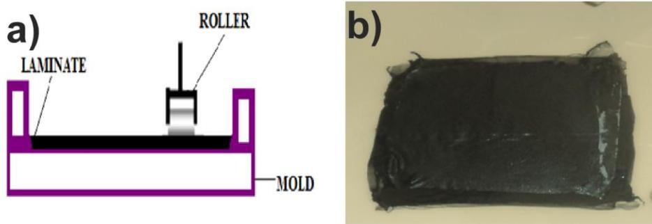
**Figure 3:** Hand lay-up method for forming the composite (a) and digital image of a flexural coupon (C<sub>1.5P</sub>) during the fabrication process (b)
