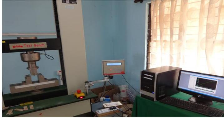
**Figure 8:** Digital image of the flexural test setup (during coupon failure)
