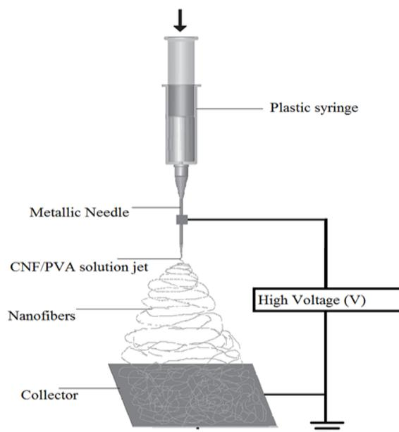
**Figure 1:** The schematic diagram of electrospinning setup describing its working mechanism
