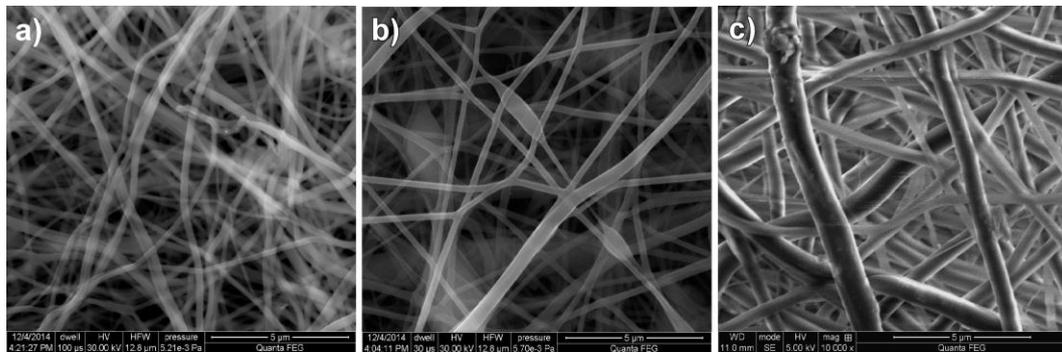
**Figure 10:** (a), (b) and (c) show the fiber morphology of C<sub>1</sub>P, C<sub>1.5</sub>P and C<sub>3</sub>P respectively.
