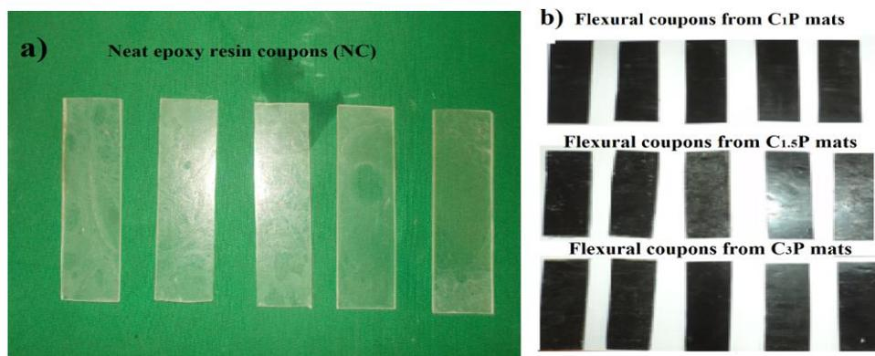
**Figure 4:** Pure epoxy resin coupons (NC) (a) and the as-fabricated CNF/PVA nanofiber mat reinforced final flexural coupons from various CNF weight percentages (b)
