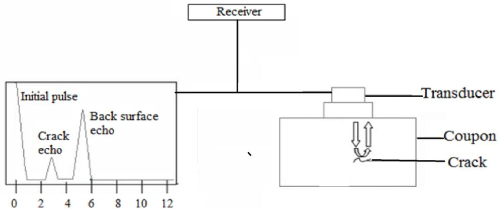
**Figure 6:** Working principle of an ultrasonic testing
