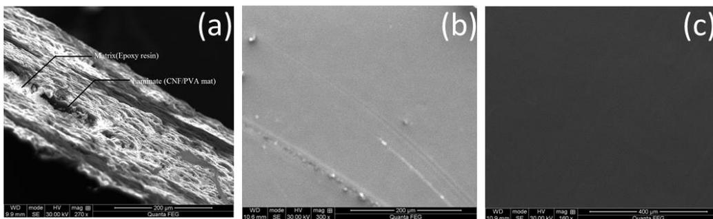
**Figure 11:** (a) The sectional view of CNF/PVA mat reinforced C<sub>3</sub>P coupon (b) Rough surface of the coupon indicating cavities and (c) Smooth surface of the coupon
