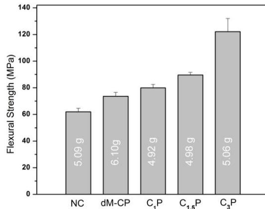
**Figure 12:** Bar diagram representing flexural strength of different composite coupons with their weight average (values indicate mean ± standard deviation)
