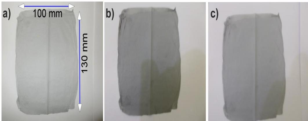
**Figure 2:** The digital images of CNF/PVA electrospun mats C<sub>1</sub>P (a) C<sub>1.5</sub>P (b) and C<sub>3</sub>P (c) (all the three samples possess the same dimension as mentioned in 'a')
