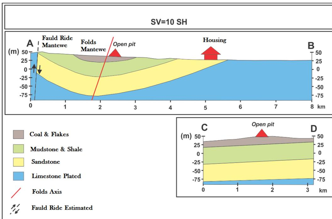
Figure 5: The profile of map of hydro-geology of the research location.
