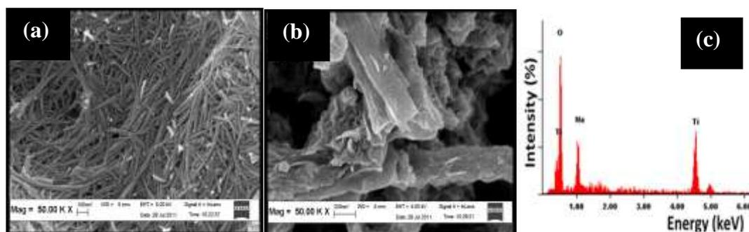
**Figure 1:** FESEM micrographs of as-synthesized samples at (a) 150 °C and (b) 200 °C (c) EDX of as-synthesized sample at 200 °C.
