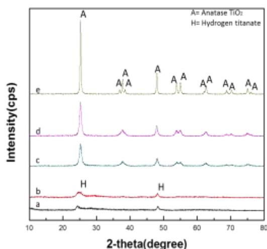
**Figure 3:** XRD patterns of (a) as-synthesized sample at 150 °C and calcined at (b) 300 °C (c) 400 °C (d) 500 °C and (e) 700 °C.
