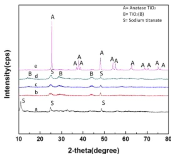
**Figure 4:** XRD patterns of (a) as-synthesized sample at 200 °C and calcined at (b) 300 °C (c) 400 °C (d) 500 °C and (e) 700 °C.
