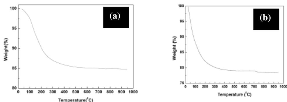
**Figure 2:** TGA themograms of as-synthesized samples at (a) 150 °C and (b) 200 °C.
