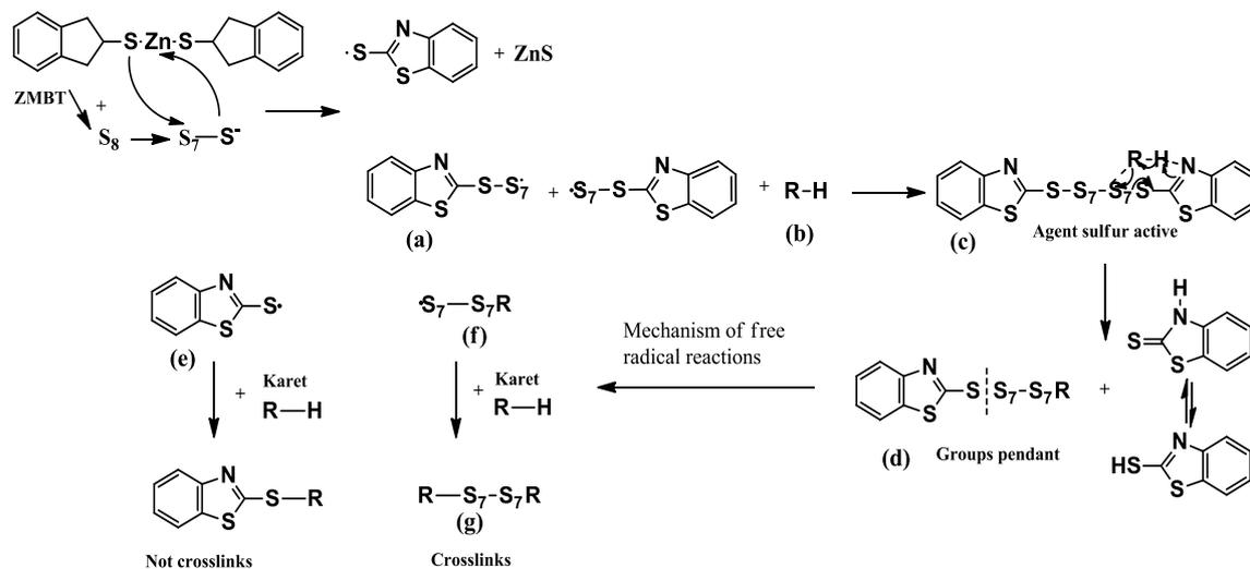
**Figure 2.** Proposed mechanisms of free radical reactions in the formation of sulfur crosslinking with rubber using accelerator and activator ZnO ZMBT
