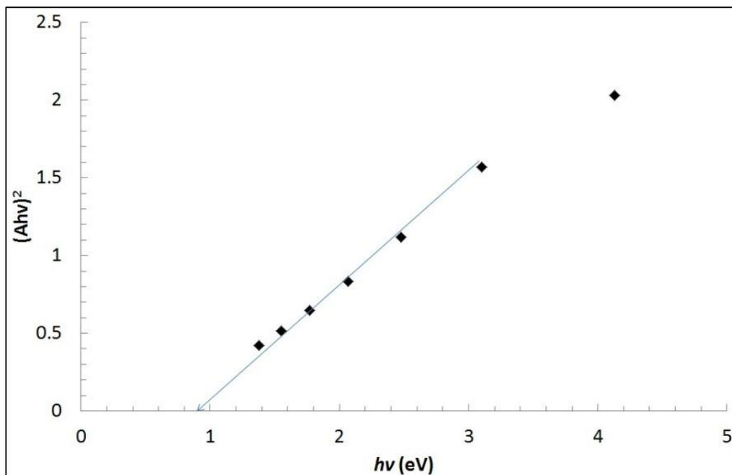
**Figure 5:** Band gap of nickel lead sulphide thin films deposited by chemical bath deposition with deposition time of 24 hours.
