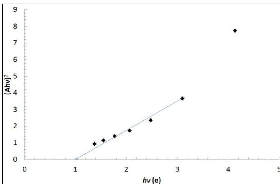
**Figure 2:** Band gap of nickel lead sulphide thin films deposited by chemical bath deposition with deposition time of 32 hours.
