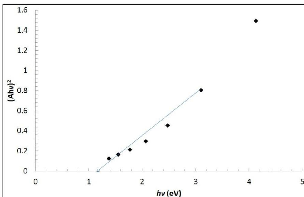
**Figure 6:** Band gap of nickel lead sulphide thin films deposited by chemical bath deposition with deposition time of 12 hours.
