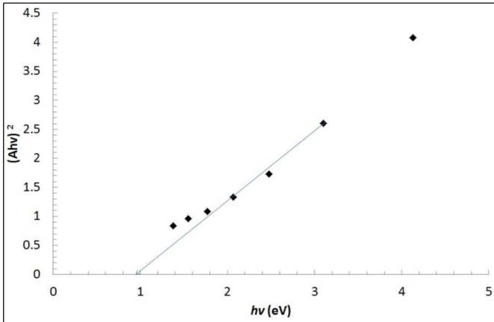
**Figure 3:** Band gap of nickel lead sulphide thin films deposited by chemical bath deposition with deposition time of 30 hours.
