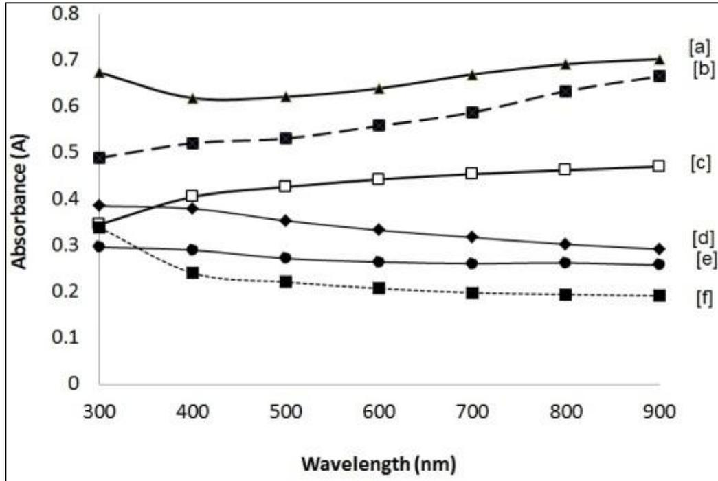
**Figure 1:** Optical absorption spectra of nickel lead sulphide thin films deposited at various deposition times. [a] 32 hours [b] 30 hours [c] 26 hours [d] 24 hours [e] 12 hours [f] 10 hours
