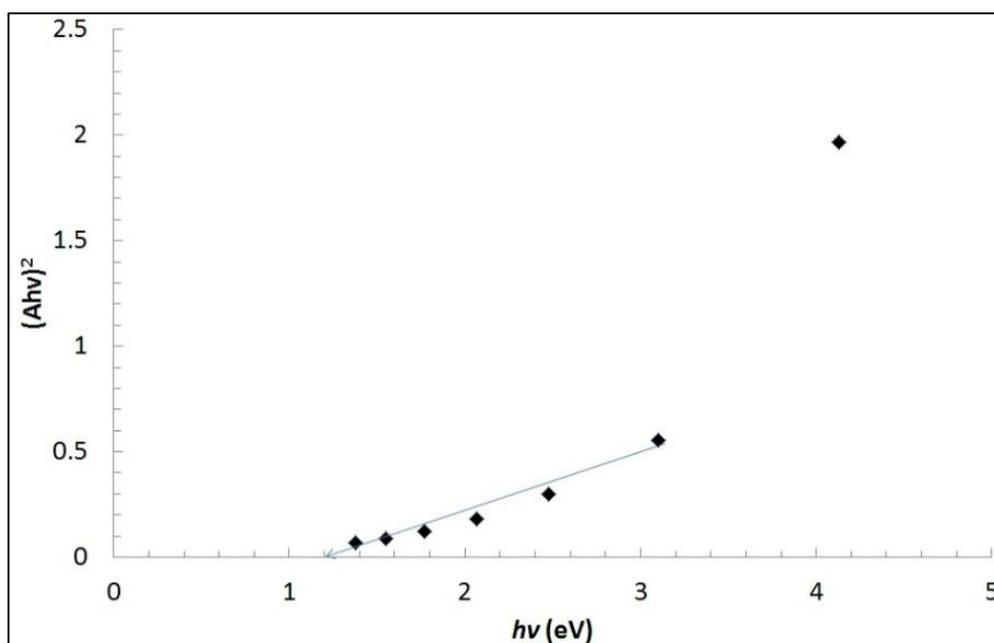
**Figure 7:** Band gap of nickel lead sulphide thin films deposited by chemical bath deposition with deposition time of 10 hours.
