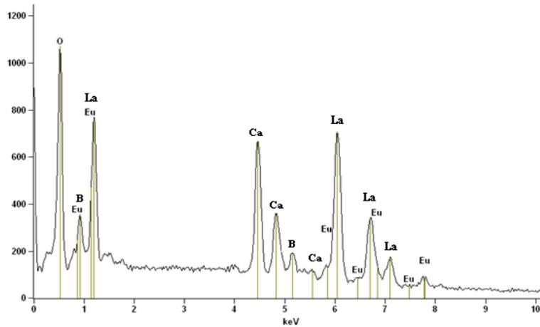
**Fig 2.** EDS of  $\text{Ca}_3\text{La}_{1.9}\text{Eu}_{0.1}(\text{BO}_3)_4$  phosphor
