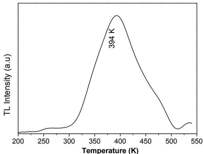
**Fig 3** TL glow curve of  $\text{Ca}_3\text{La}_{1.9}\text{Eu}_{0.1}(\text{BO}_3)_4$  phosphor
