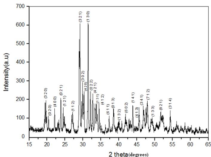
Fig 1 XRD of  $\text{Ca}_3\text{La}_{1.9}\text{Eu}_{0.1}(\text{BO}_3)_4$  phosphor
