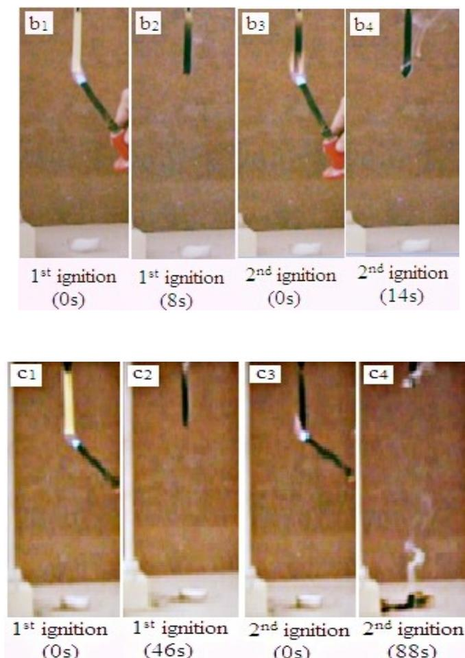
**Figure 2:** UL-94 VB test images of (a) phospho-EP<sub>1NC</sub>, (b) phospho-EP<sub>2NC</sub>, and (c) phospho-EP<sub>3NC</sub> samples
