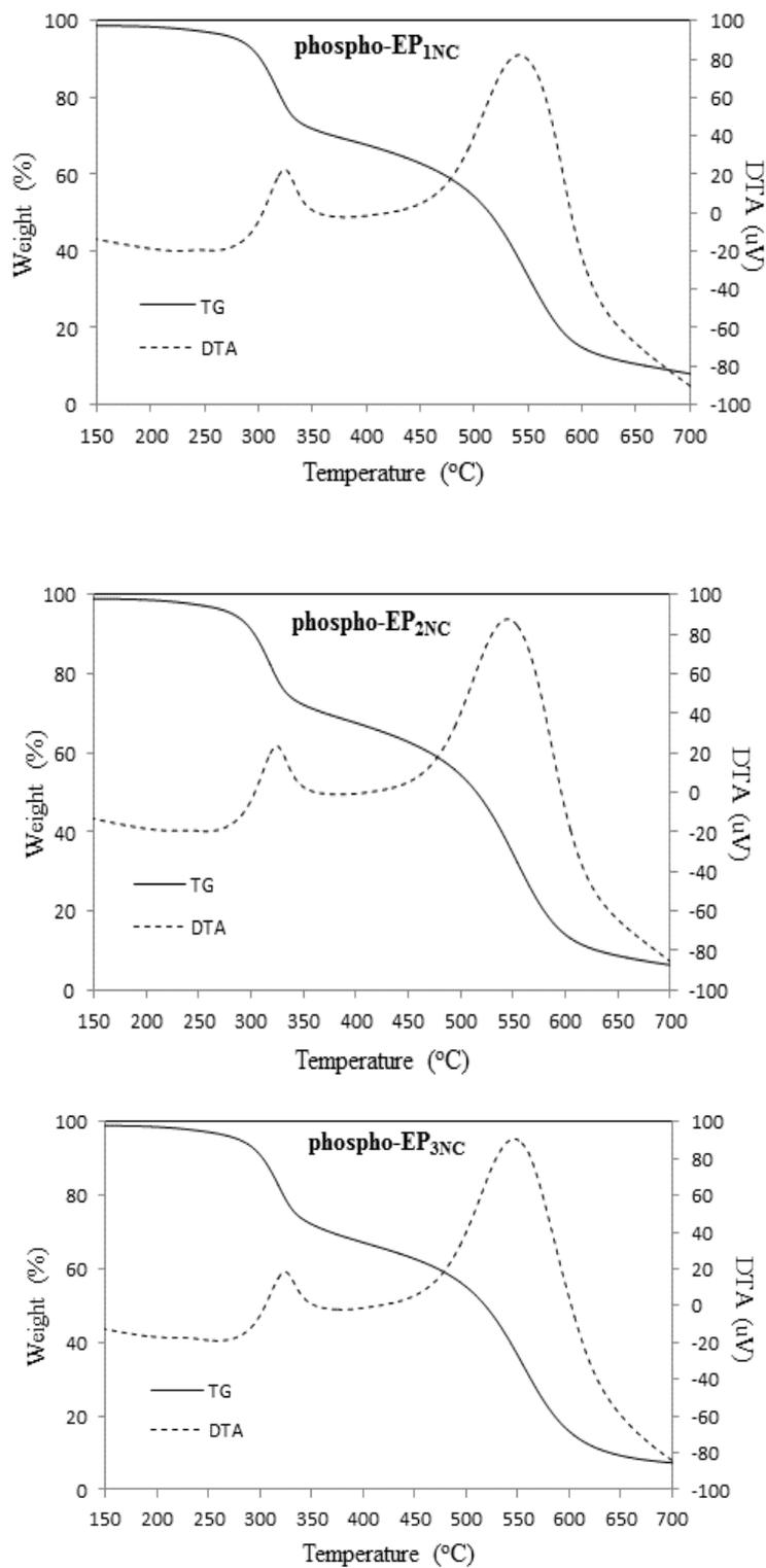
**Figure 1:** TG-DTA thermograms of phosphorylated epoxy samples
