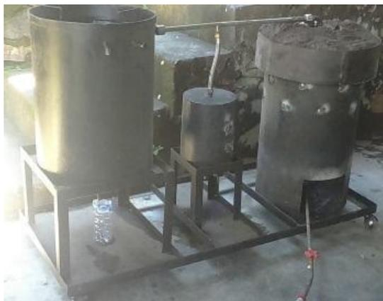
Figure 1. Pyrolysis reactor
