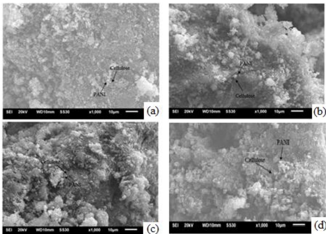
**Figure 7.** SEM micrograph of 1000x magnification (a) PANI-Cellulose Composite without Swelling and sonication (b) Swelling and Sonication methods (c) Swelling method (d) Sonication method
