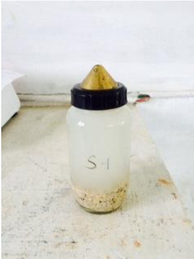
Fig.3.1. Specific gravity test of CCS
