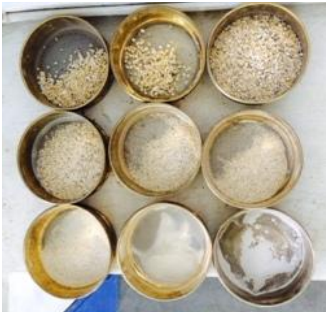
Fig.3.2. Fineness modulus test of CCS
