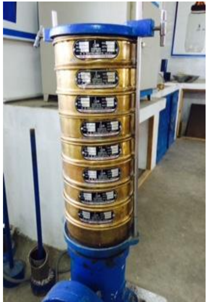
Fig.4.2 Sieve analysis of CCS
