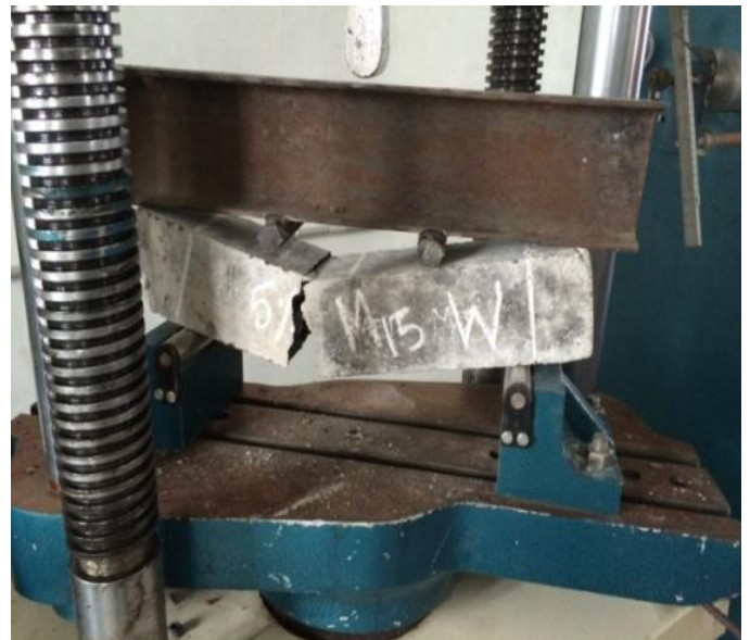
Fig.4.7. Flexural Test specimen
