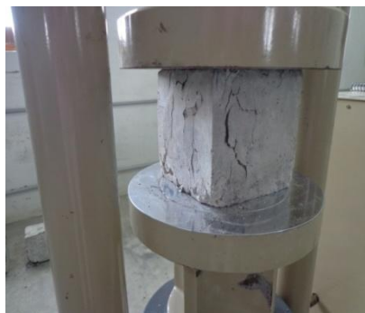
Fig.4.5. Compressive test specimen
