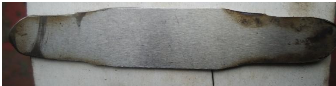
Fig3. Worn out valve
