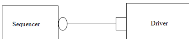
Figure 3.3: TLM communication between Sequencer and Driver
