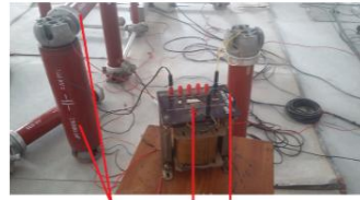
Fig (2.2.4)Transformer under test (1-Ø, 1KVA, 240V/240V transformer)
