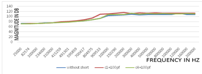
Fig (3.1.5) switching impulse voltage based transfer function analysis-axial deformation
