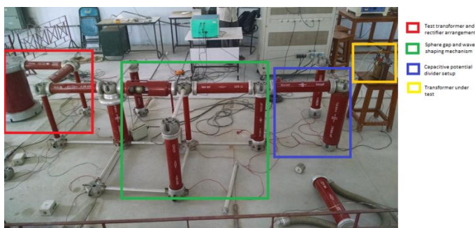
Fig (2.2.3) LIFRA setup for testing of 1-Ø, 1KVA, 240V/240V transformer
