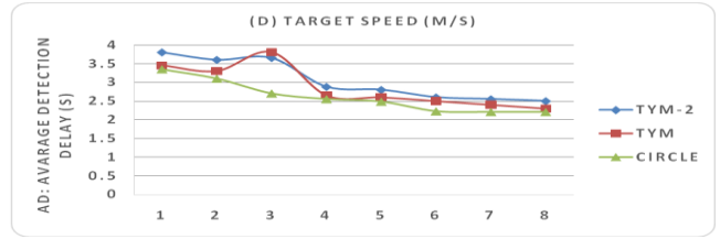
Figure: 6 (d) Performance under various target speeds w.r.t average detection delay (Target speed vs. Average detection delay).
