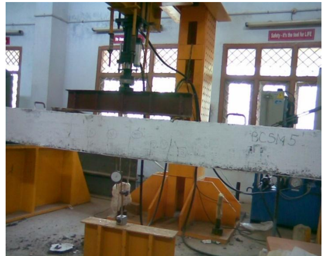
Fig. 4 Experimental set up for cyclic loading The load imposed on each beam and the experimental results (deflections at failure) are given in the Table 4
