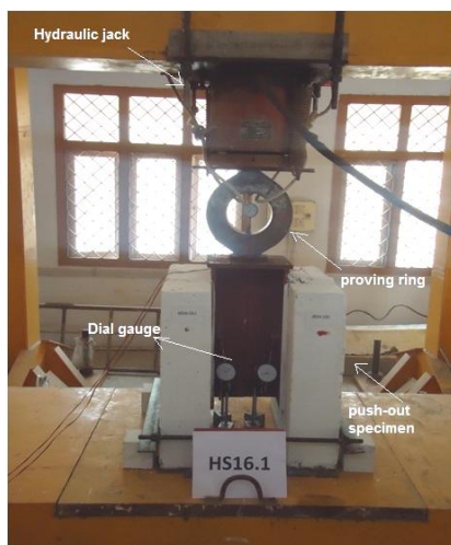
Fig.5 Test setup and instrumentation
