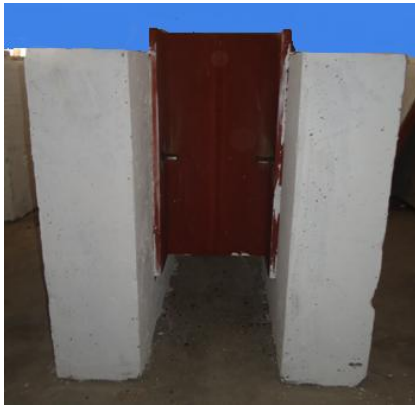
Fig.5 Full-scale push – out specimen after welding
