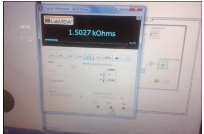
Fig. 6. Result for resistance in an current transformer measured using NI-ElvisII+
