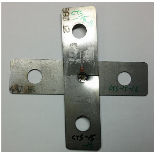
(c) Fatigue Fractured Specimen
