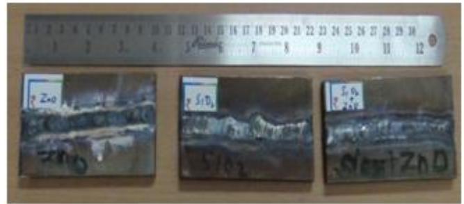
Fig.1. Photograph view of the bead on plate welds
