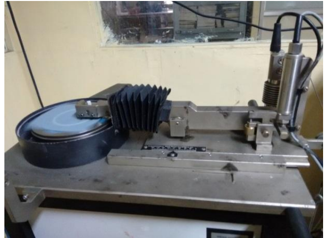
Fig.1. Pin on disc wear tester
