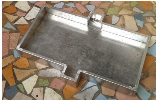
Figure 2: Fabricated Body of The Robot
