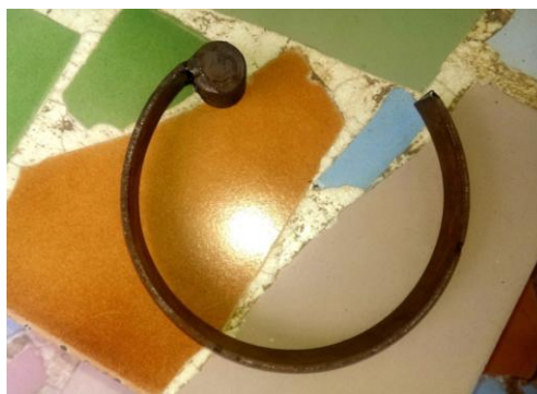
Figure 4: Fabricated Leg of The Robot
