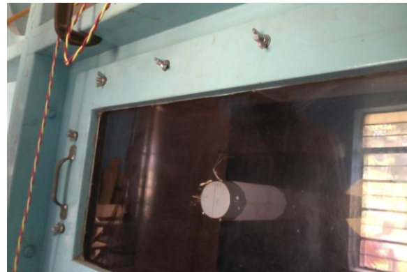
Figure 4: Roughness Cylinder At Test Rig
