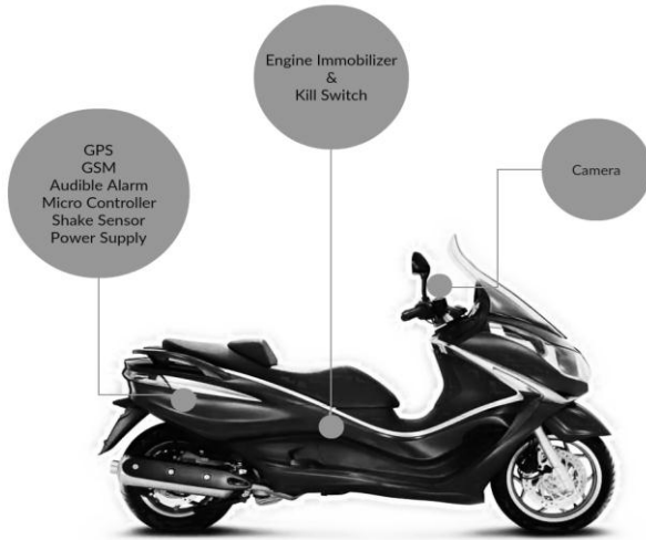
Figure 7. Hardware Installation of Motorcycle Theft Prevention and Recovery Security System
