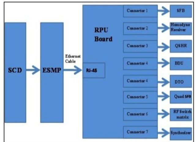
Figure 1. System level block diagram
