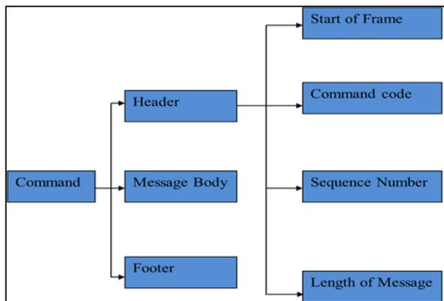
Figure 3: Command Frame Format
